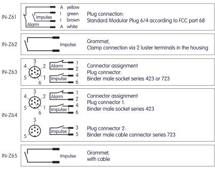
A: Alarm contact, reed switch (normally closed) I: Totalizing contact, reed switch (normally open)
